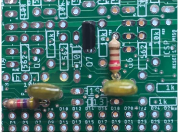
You can also see in the above picture where the 4.7k ohm resistor R16 mounts (bottom left of picture) as the printing was interrupted by a via.
