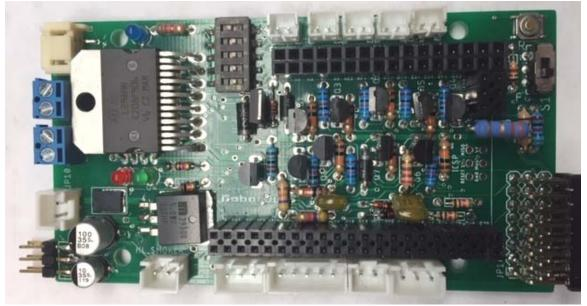
Install the Arduino pin receptacles last, since they melt really easy when touched by a soldering iron. I recommend assembling the Arduino, its pins, the receptacles and the board all together before soldering any of it, so the pins will align correctly. Solder the pins/receptacles sporadically around the perimeter on both sides before doing final soldering, which ensures no warping. Remove the Arduino after final soldering to ensure all pins will align when reinstalling it.
