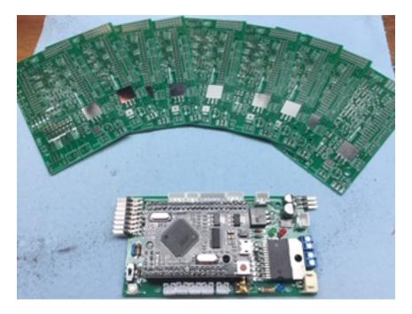
Here is the FatFingersV2 boards, one fully assembled with the Arduino installed and the remaining 9 boards not yet started. These are from Seed, but be aware that shipping took 3 months from China. OSH makes them here in the US, but they are more expensive, and didn't offer the thicker laminate (1.6mm). Of course there are many makers of prototype boards out there, so just do a web search and decide which fits your budget and time frame.
