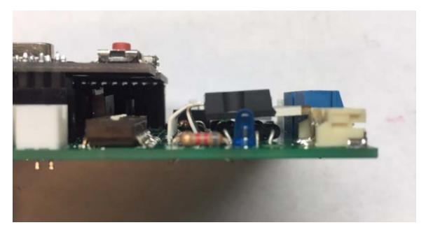
Install the two screw terminals next so you can judge how much to bend the pins of the motor controller so it will sit fully flat as above.
